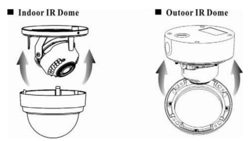
Reinstall the indoor dome cover and the main body by turning the dome clockwise until it locks into place
